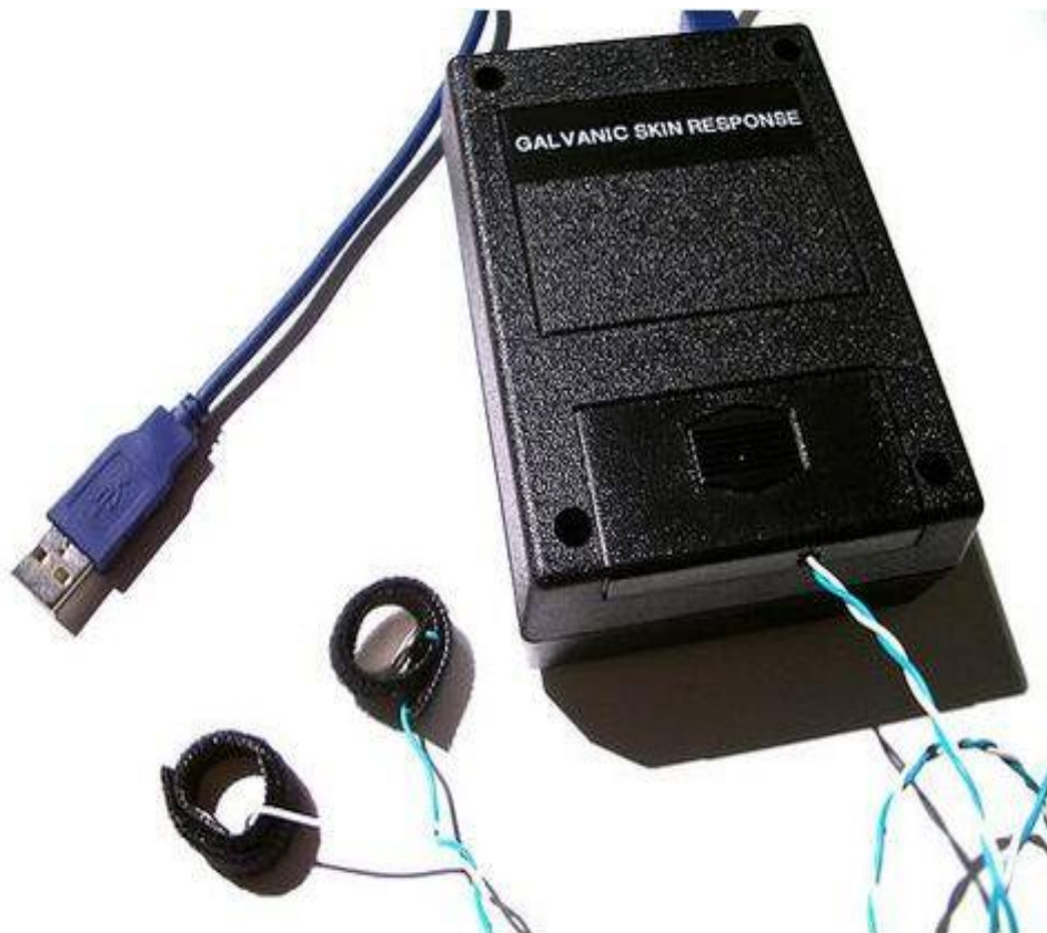
Fig 1: Shows a typical setup for measuring GSR. The sensor is just a 9V LEGO motor wire and some aluminum foil wrapped around your fingers with tape. A small current is generated in a pocket size amplifier which is able to sense fluctuations upto a few microsiemens.
