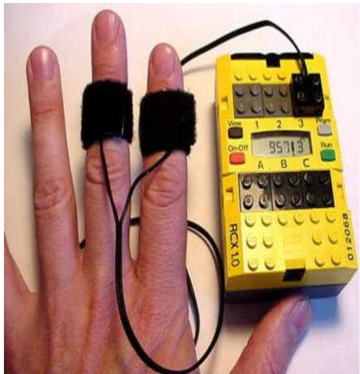
Fig 3: A simple LEGO setup for a lie detector test
