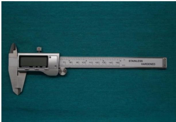
Fig 2: Vernier Calliper
